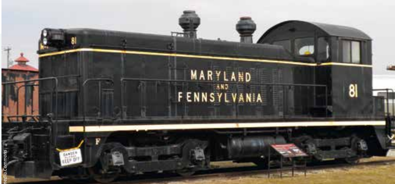
Maryland and Pennsylvania locomotive No. 81 (1946), an EMD NW2 at the Railroad Museum of Pennsylvania. One of the the first diesel electrics to see widespread use.
