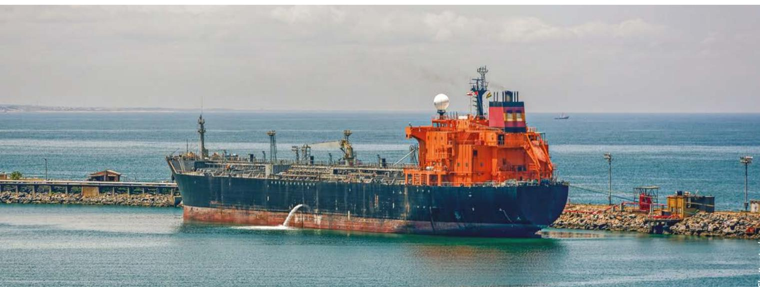
Crude oil tanker pumping ballast water in Lagos, Nigeria.
